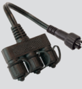
Cablesplitter (6006011) Cable splitter 15 cm SPT-2W 16AWG (with 3 connectors)
