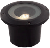
Rubum (3159011) Warm white 3,5 W / 280 lumen Aluminium - Black 110 x 155 mm (H x Ø) Including ground tube Drillhole 120 mm
